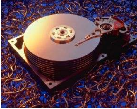
This Barracuda hard disk has 10 platters.
